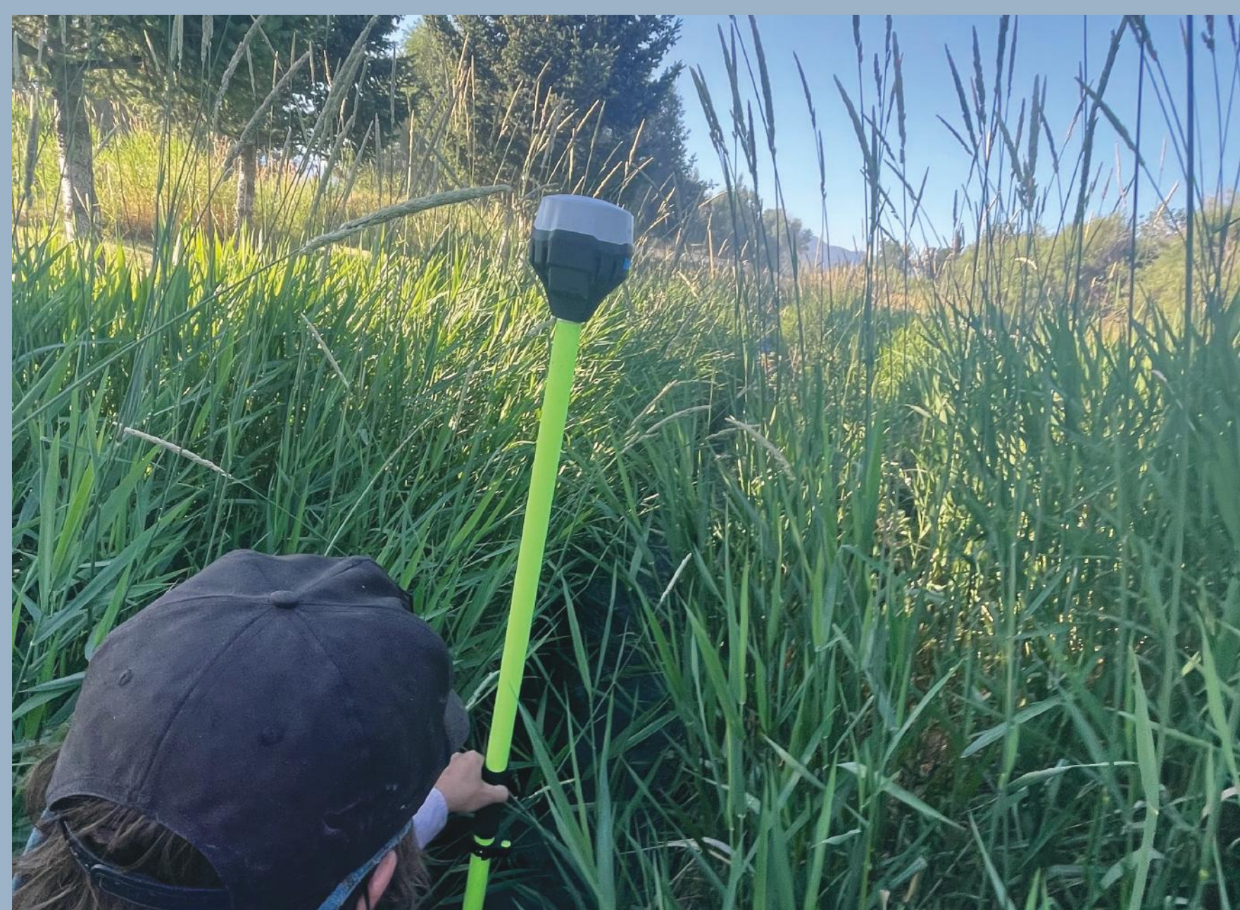
Groundtruthing the course of an unnamed irrigation ditch using an Emlid Reach RS2 GPS Receiver
