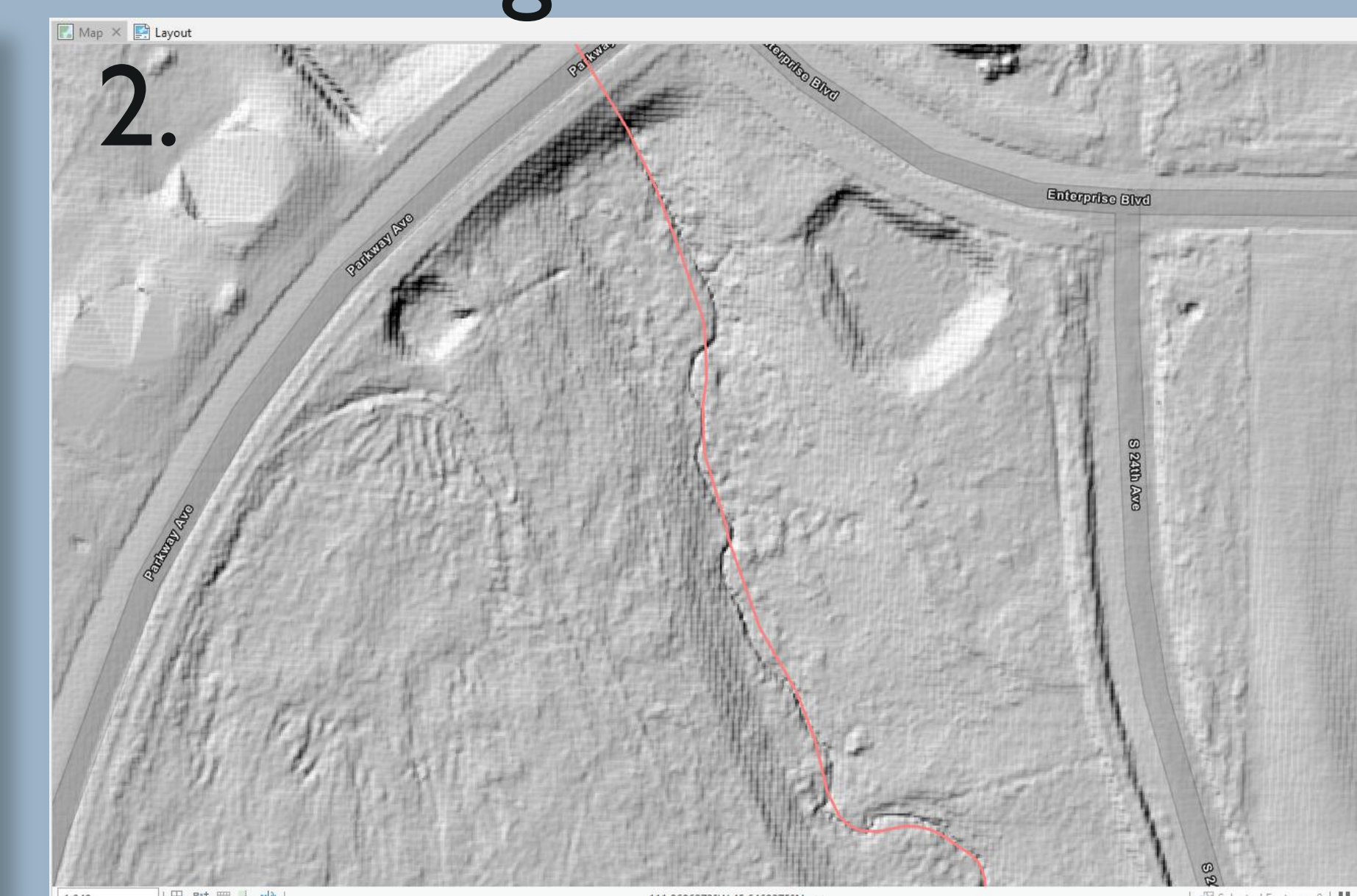
Line segment overlaid with 2018 LiDAR revealing waterway sections obscured by tree cover and other vegetation
